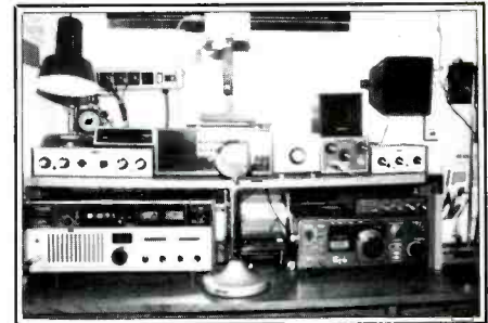
Here's the neat, multi-mode listening post of Frank Mierzwinski in Pennsylvania, including a Kenwood R-1000 SW receiver, also an SSB transceiver for 27 MHz.
