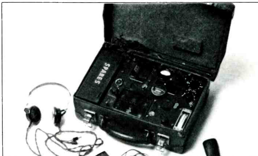
A WWII British spy and saboteur transceiver constructed in a suitcase.
